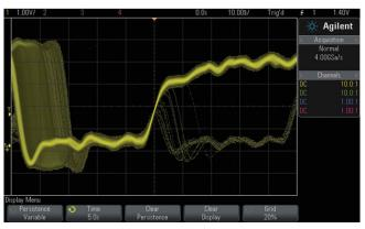
Figure 3: The Agilent MSO/DSO3000 X-Series oscilloscope reliably captures the infrequently occurring metastable state while updating at 1,000,000 waveforms per second.
